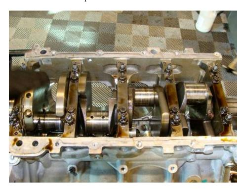
The damage report is as follows: I spun bearings #5 and 6; #7 was on its way out.
