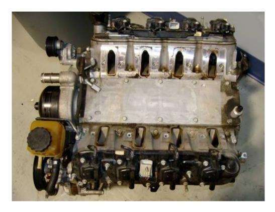
Unlike some other motors you can't get to the lifters by removing the intake. You actually have to remove the heads to get to them.
